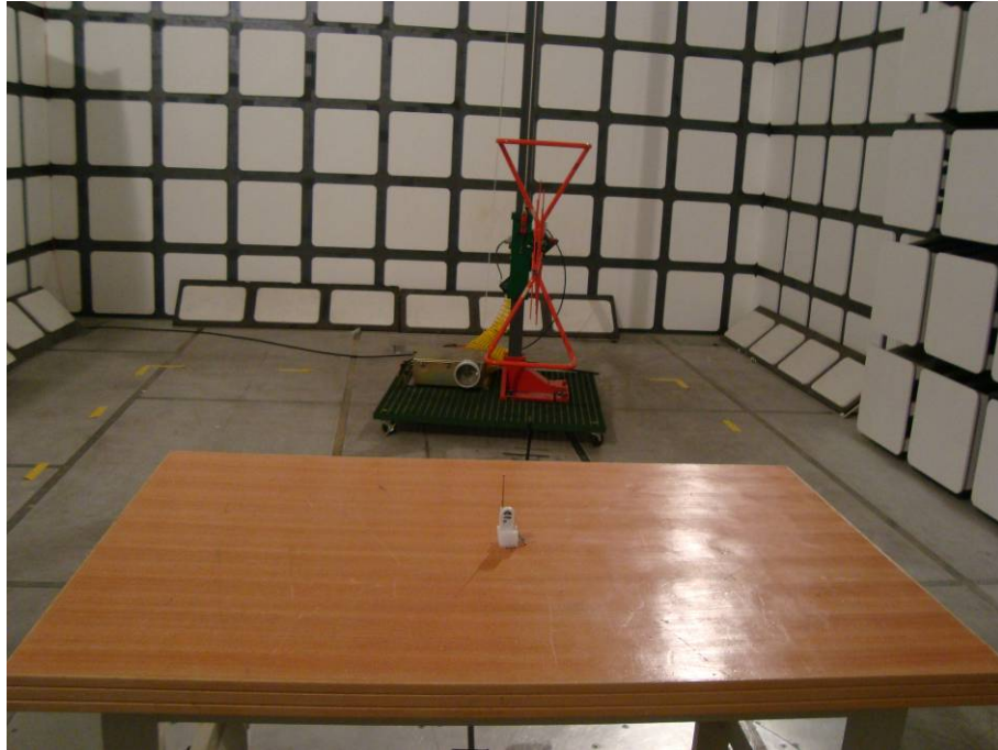
Radiated Emission – Stand Rear View (Below 1GHz)
