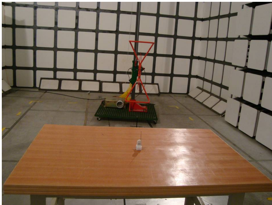
Radiated Emission – Stand Rear View (Below 1GHz)
