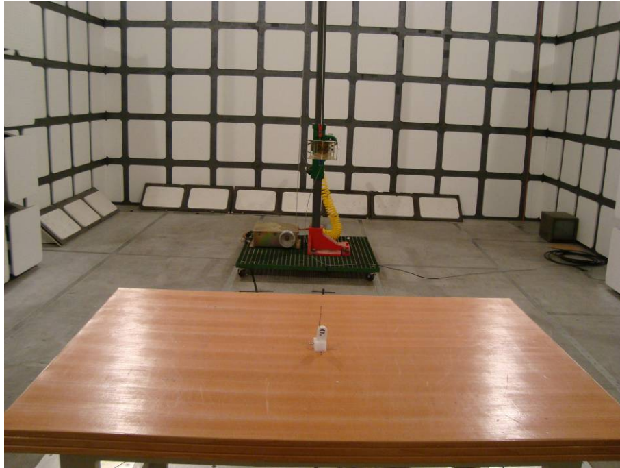
Radiated Emission – Stand Front View (Above 1GHz)
