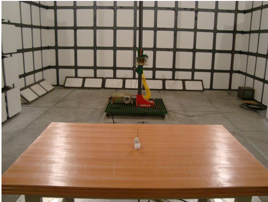
Radiated Emission – Stand Rear View (Above 1GHz)
