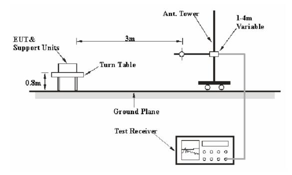
The deactivation test was performed in the 3 meters chamber B test site, using the setup accordance with the ANSI C63.4 - 2003. The specification used was the FCC 15.231(a) limits.
