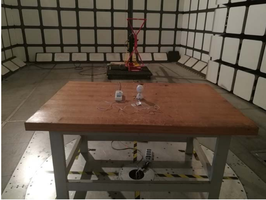
Radiated Emissions View (Below 1 GHz)
