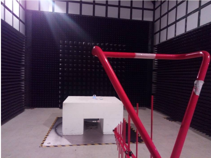
Radiated Emissions Tested View (Below 1GHz)
