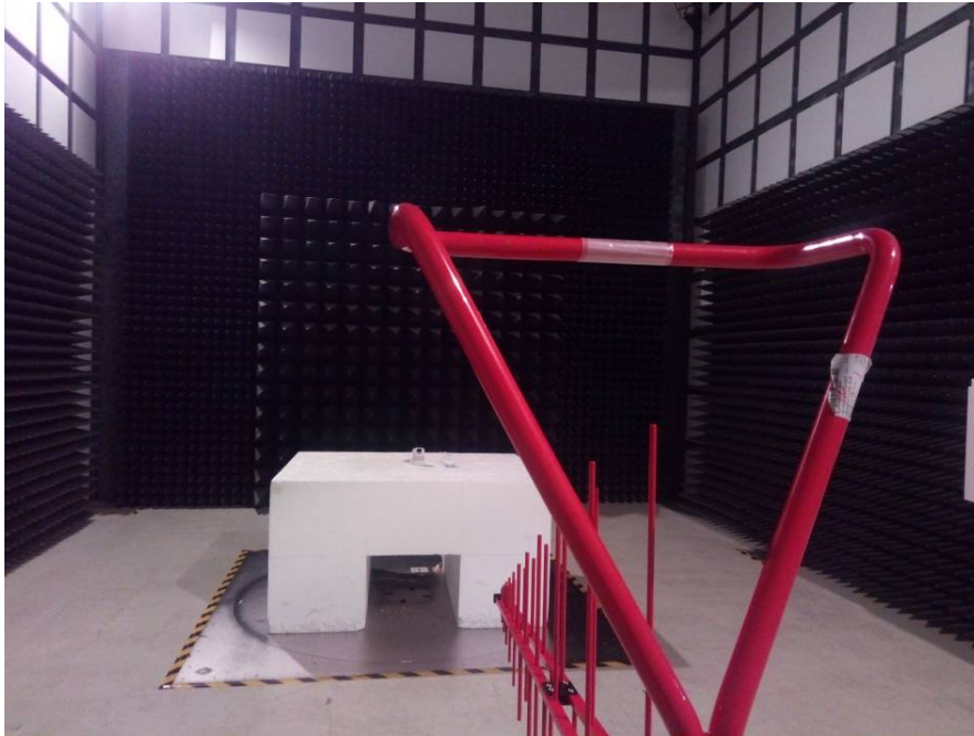
Radiated Emissions Tested View (Below 1GHz)
