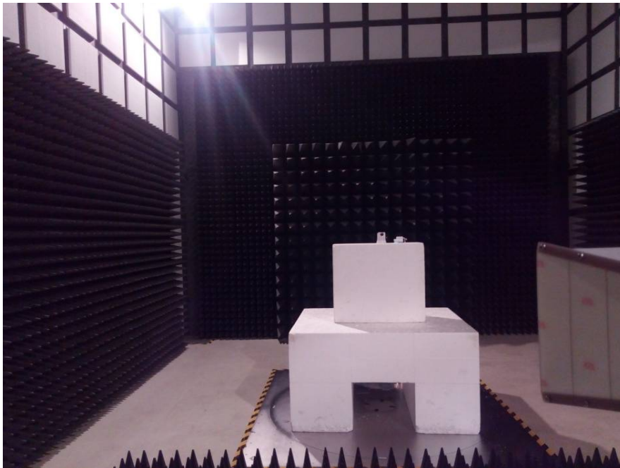
Radiated Emissions Tested View (Above 1GHz)
