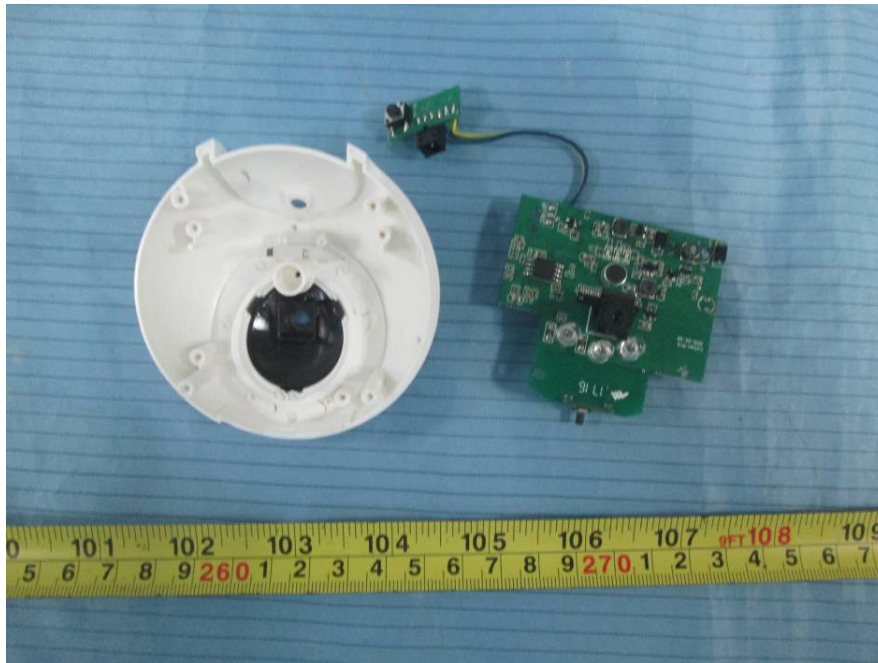
EUT- Cover off View 6
