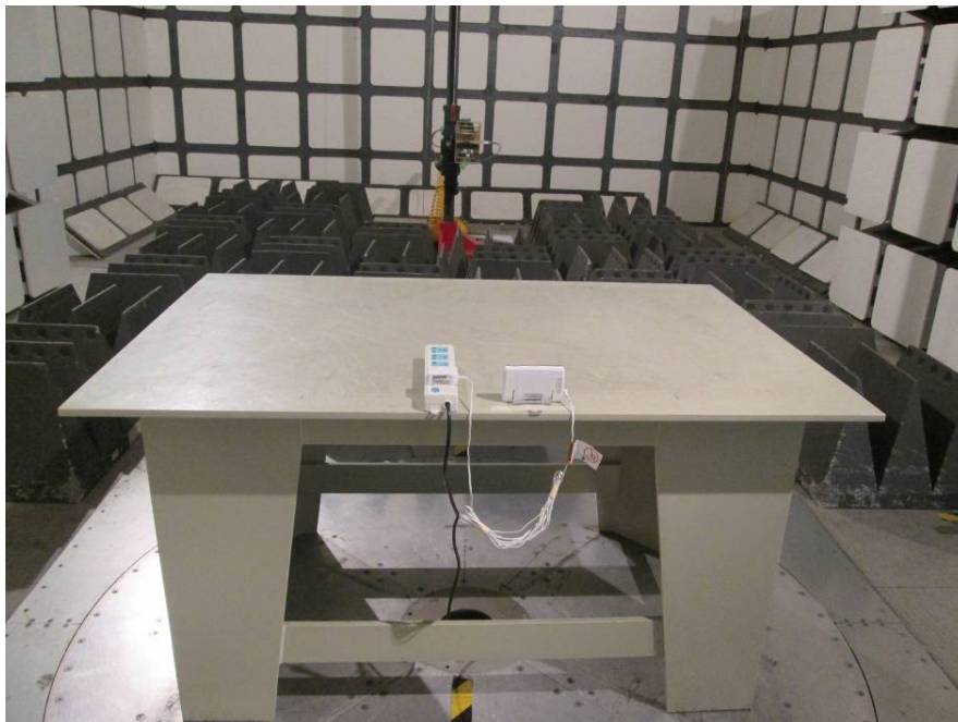
Radiated Emissions – Rear View (1-25 GHz)
