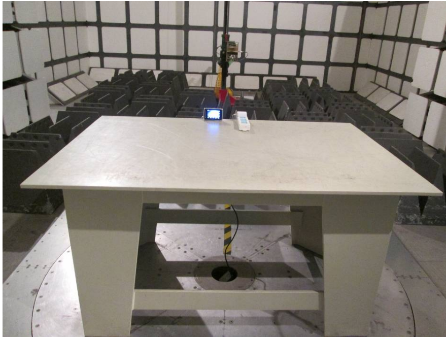
Radiated Emissions – Front View (1-25 GHz)
