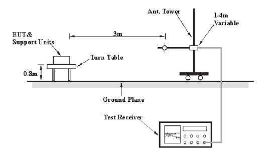
The radiated emission tests were performed in the 3 meters test site, using the setup accordance with the ANSI C63.4-2009. The specification used was the FCC 15.209 and FCC 15.247 limits.
