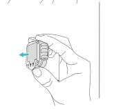
3. Slide camera onto mount until it clcks into place.
