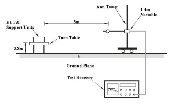
The radiated emission tests were performed in the 3 meters chamber B test site, using the setup accordance with the ANSI C63.4-2003. The specification used was the FCC 15.209 and FCC 15.247 limits.
