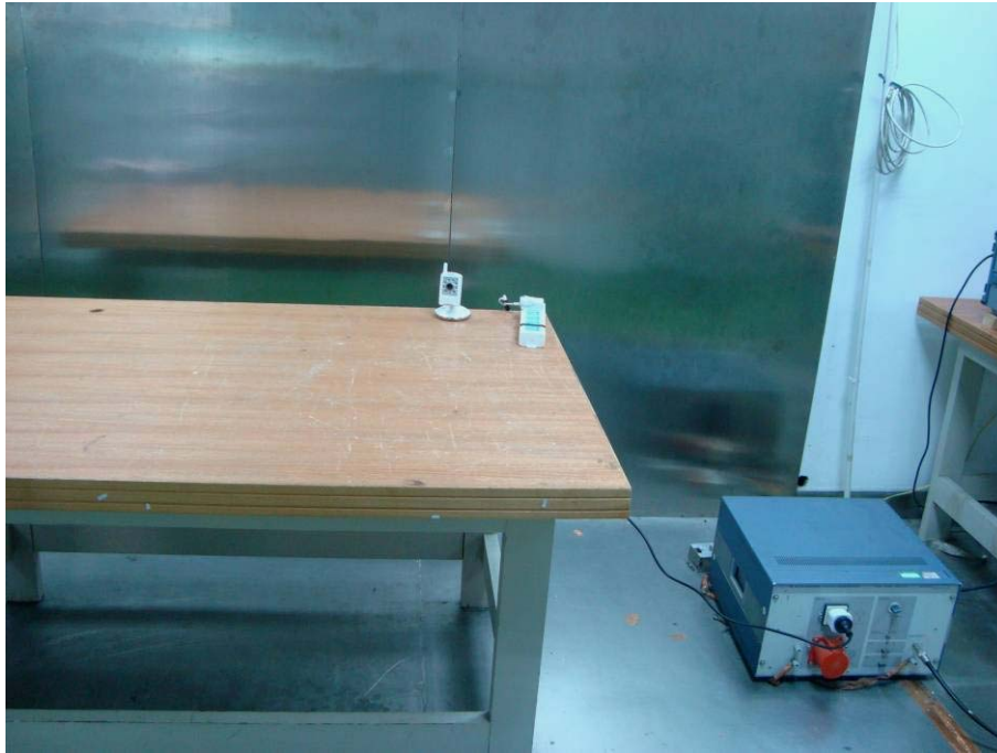
AC Line Conducted Emissions - Side View
