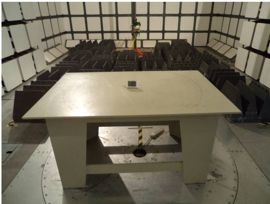
Radiated Emissions – Rear View (1-25 GHz, Powered by battery)
