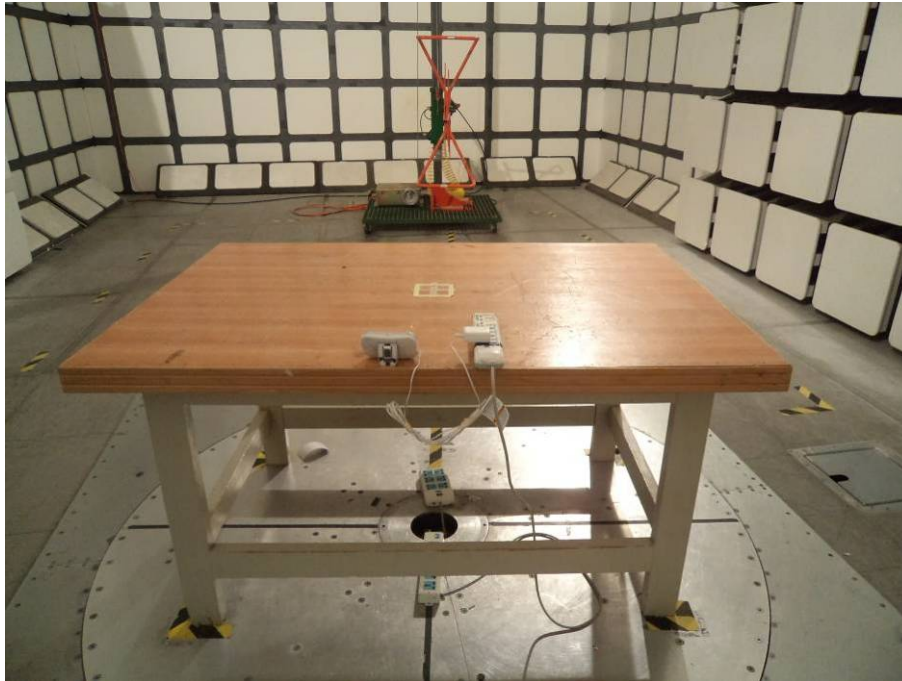
Radiated Emissions View (30-1000 MHz, Powered by adapter)
