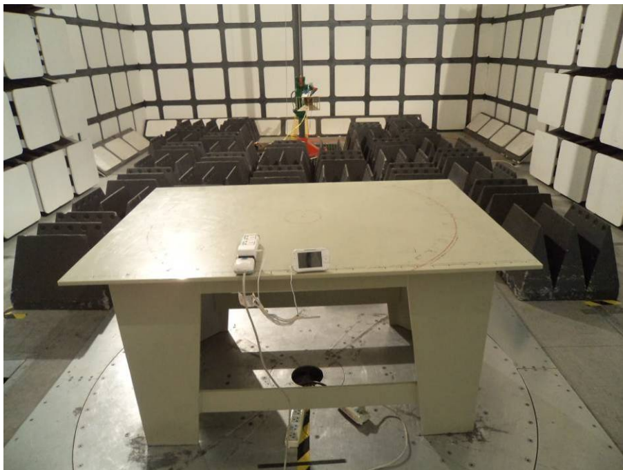
Radiated Emissions – Rear View (1-25 GHz, Powered by adapter)
