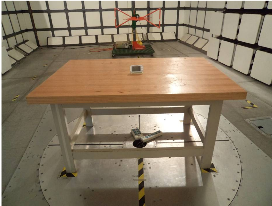
Radiated Emissions View (30-1000 MHz, Powered by battery)
