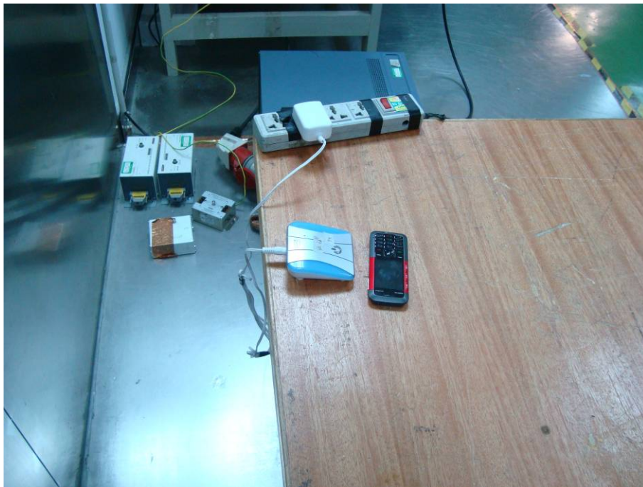
AC Line Conducted Emissions - Side View
