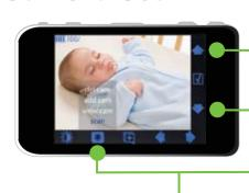
To scan all cameras in use for 8 second intervals, press camera button from the touch menu. Use the **up and down** arrows to navigate to the scan option. Press **select** to enter the scan mode.
