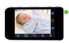
The monitor will automatically scan through all camera options every 8 seconds. To stop scan mode at anytime press the **home** button. If **scan mode** stops on an undesired camera selection, press **camera** button from touch menu and select **view camera** option. Follow directions above listed in view camera.
