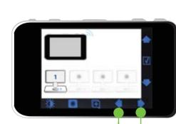
Use the **left and right** arrows t highlight the camera you would like to delete and **press select** to delete that camera. To exit hit the home key
