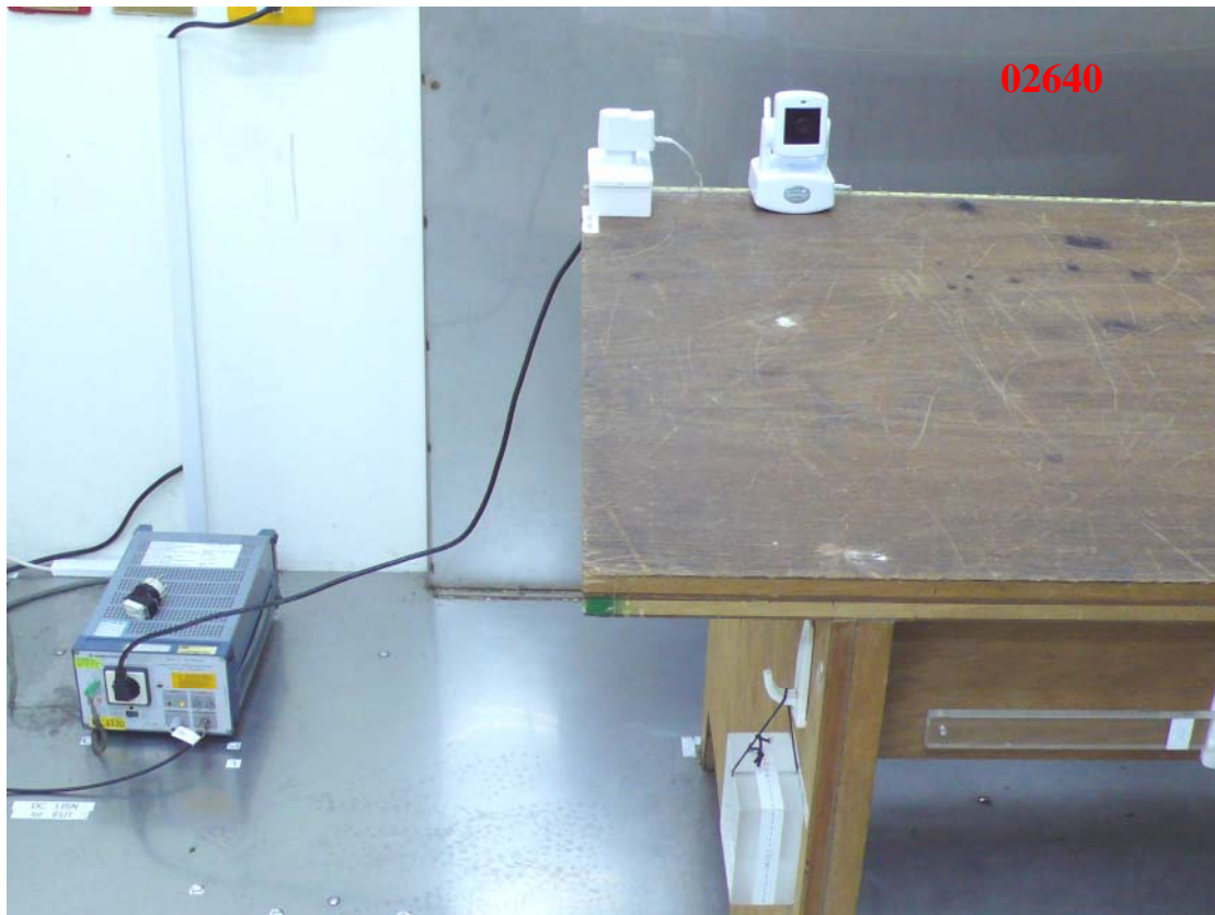
Photo 1: Conducted Emission Test Set-up photo
