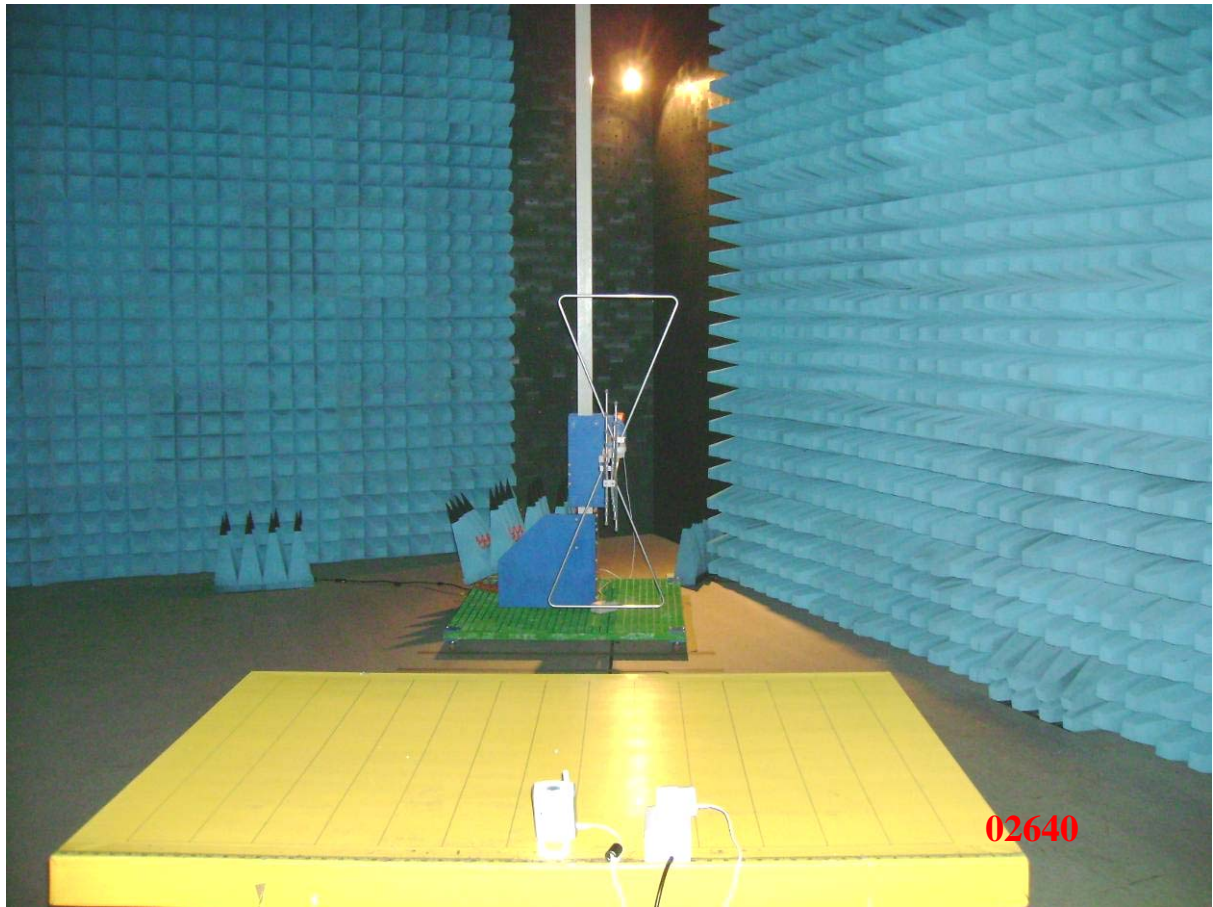
Photo 2: Radiated Emission Test set-up photo
