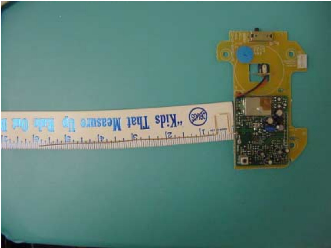
Main board, with RF board showing antenna length.
