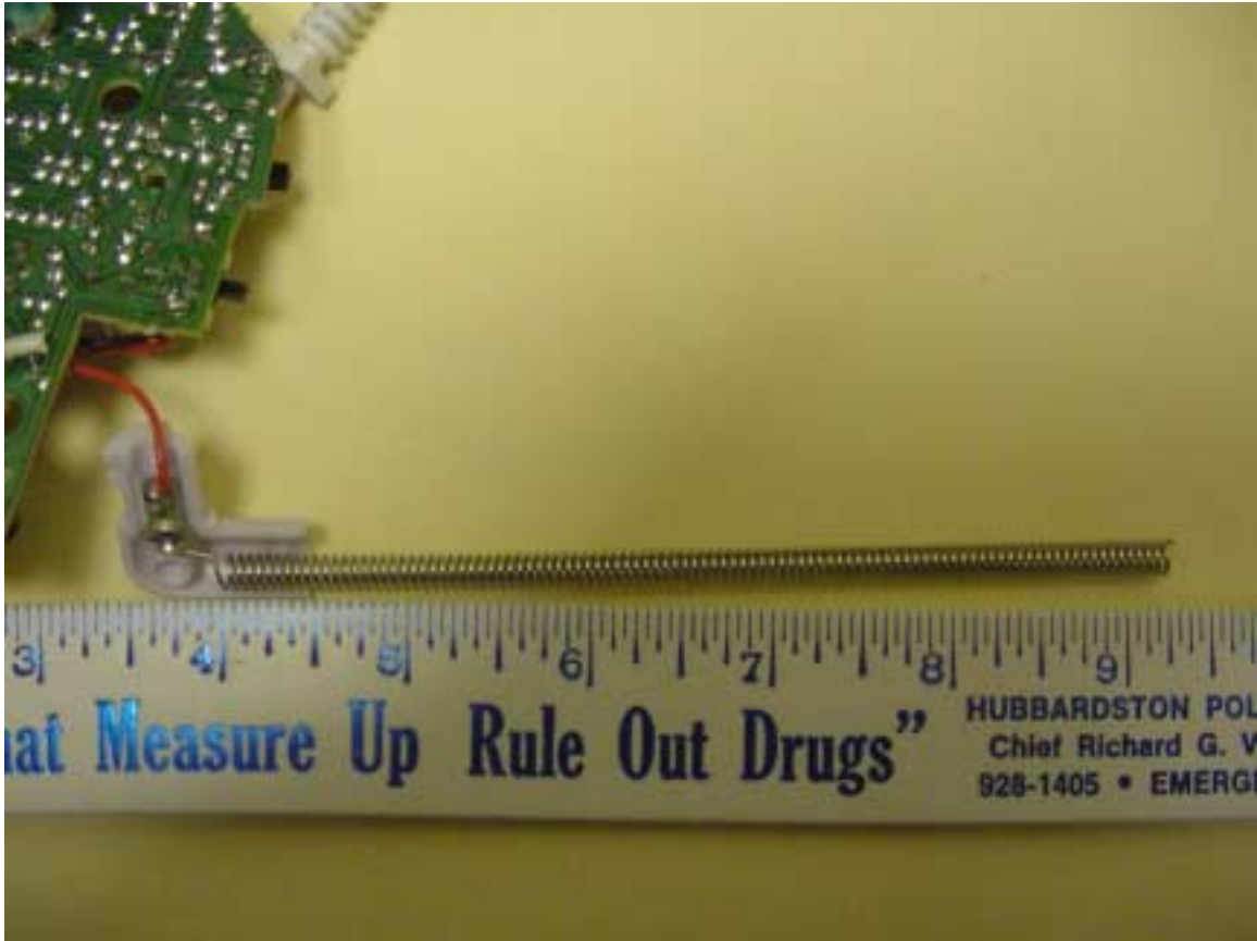
Antenna and connection
