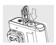
Insert 2xAA or LR6 batteries, make sure the "+" and "-" battery contacts are properly oriented, push down the cover and slide it back.
