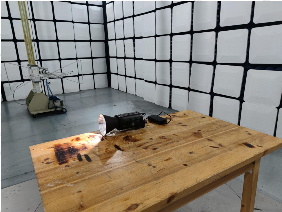
Photo of Radiation Emission Test
