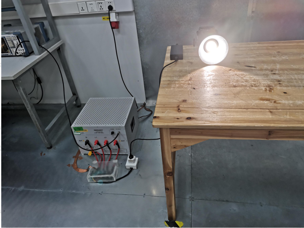
Photo of Conducted Emission Measurement
