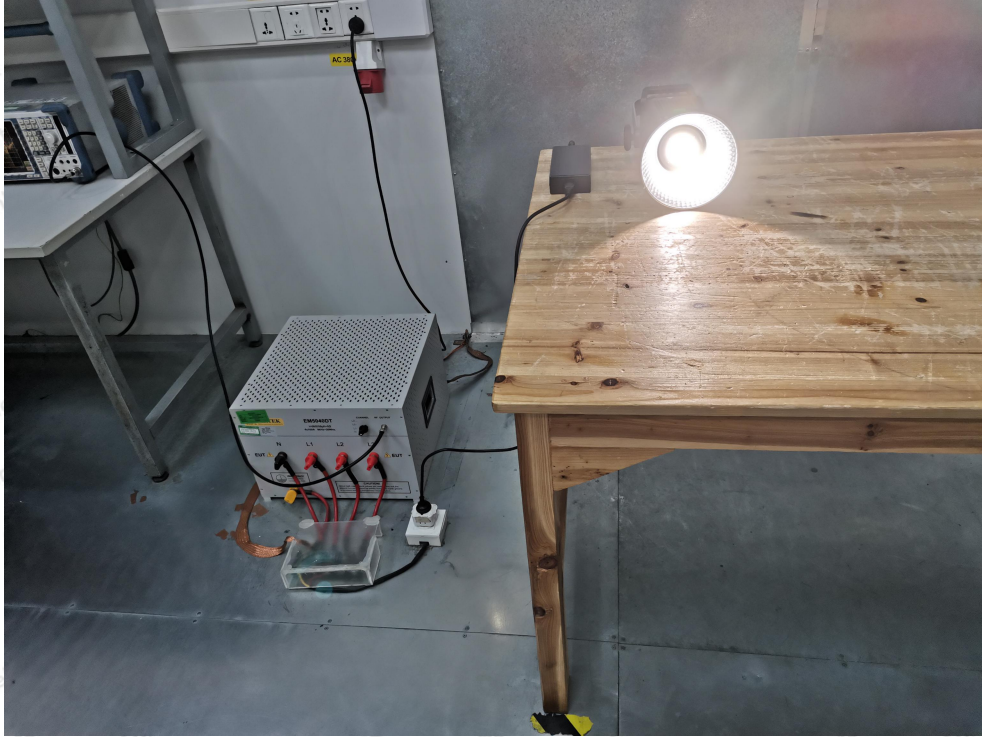
Photo of Conducted Emission Measurement
