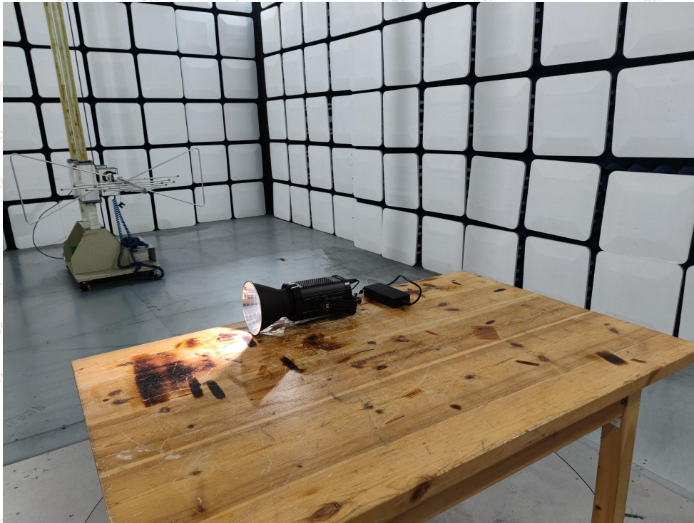
Photo of Radiation Emission Test
