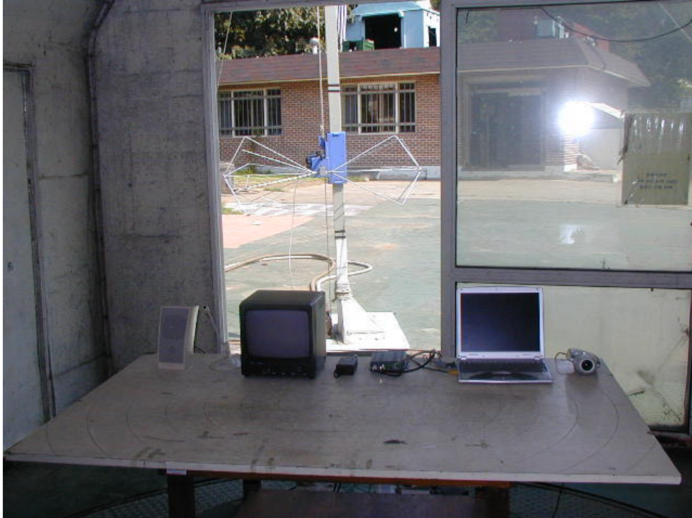
RADIATED EMISSION SETUP PHOTOGRAPH - FRONT VIEW ( 30 - 300 MHz )
