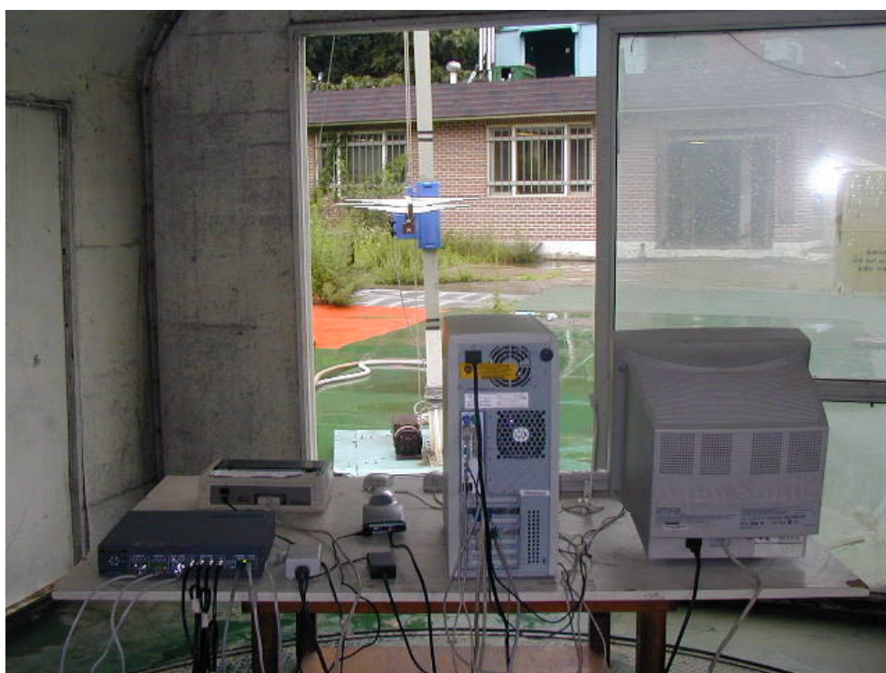
RADIATED EMISSION SETUP PHOTOGRAPH - REAR VIEW ( 300 - 1000 MHz )
