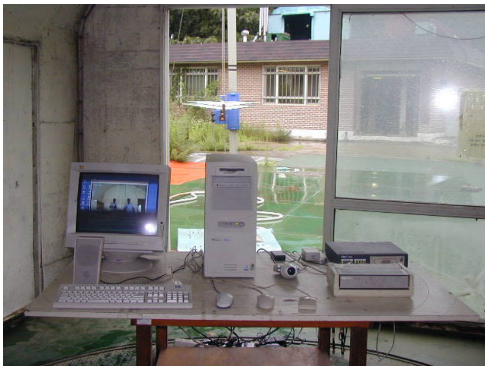
RADIATED EMISSION SETUP PHOTOGRAPH - FRONT VIEW ( 300- 1000 MHz )
