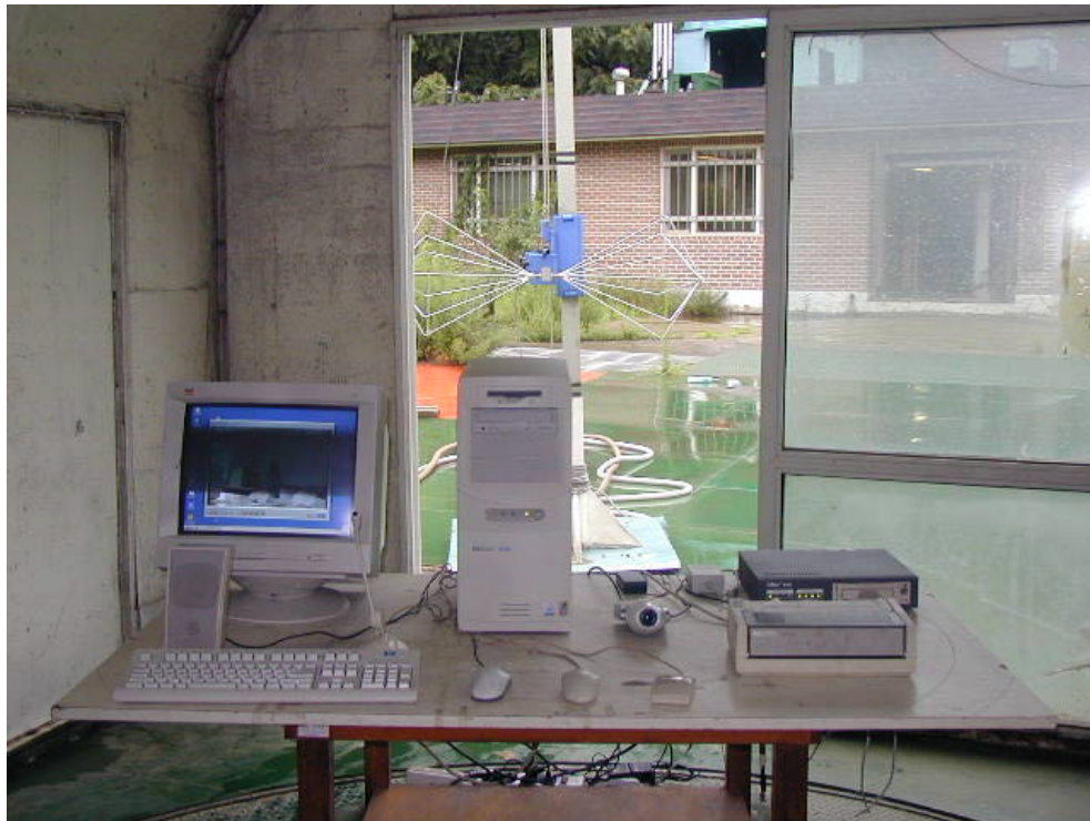
RADIATED EMISSION SETUP PHOTOGRAPH - FRONT VIEW ( 30 - 300 MHz )
