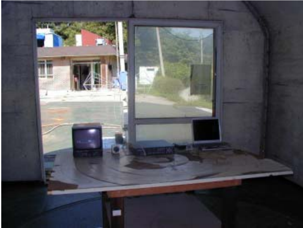
RADIATED EMISSION SETUP PHOTOGRAPH - FRONT VIEW ( 30 - 300 MHz )
