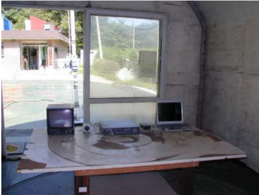
RADIATED EMISSION SETUP PHOTOGRAPH - FRONT VIEW ( 300- 1000 MHz )
