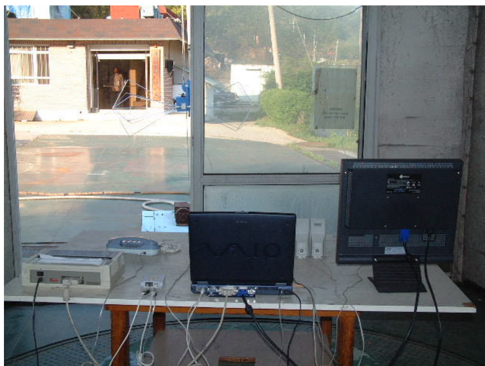
RADIATED EMISSION SETUP PHOTOGRAPH - REAR VIEW ( 30 - 300 MHz )
