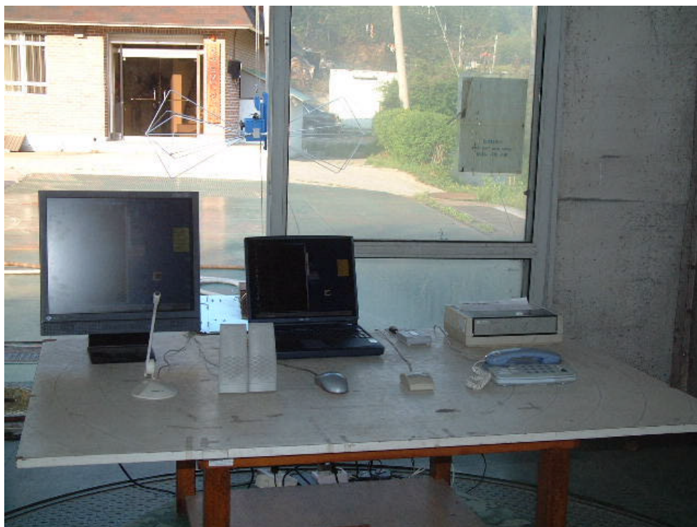
RADIATED EMISSION SETUP PHOTOGRAPH - FRONT VIEW ( 30 - 300 MHz )
