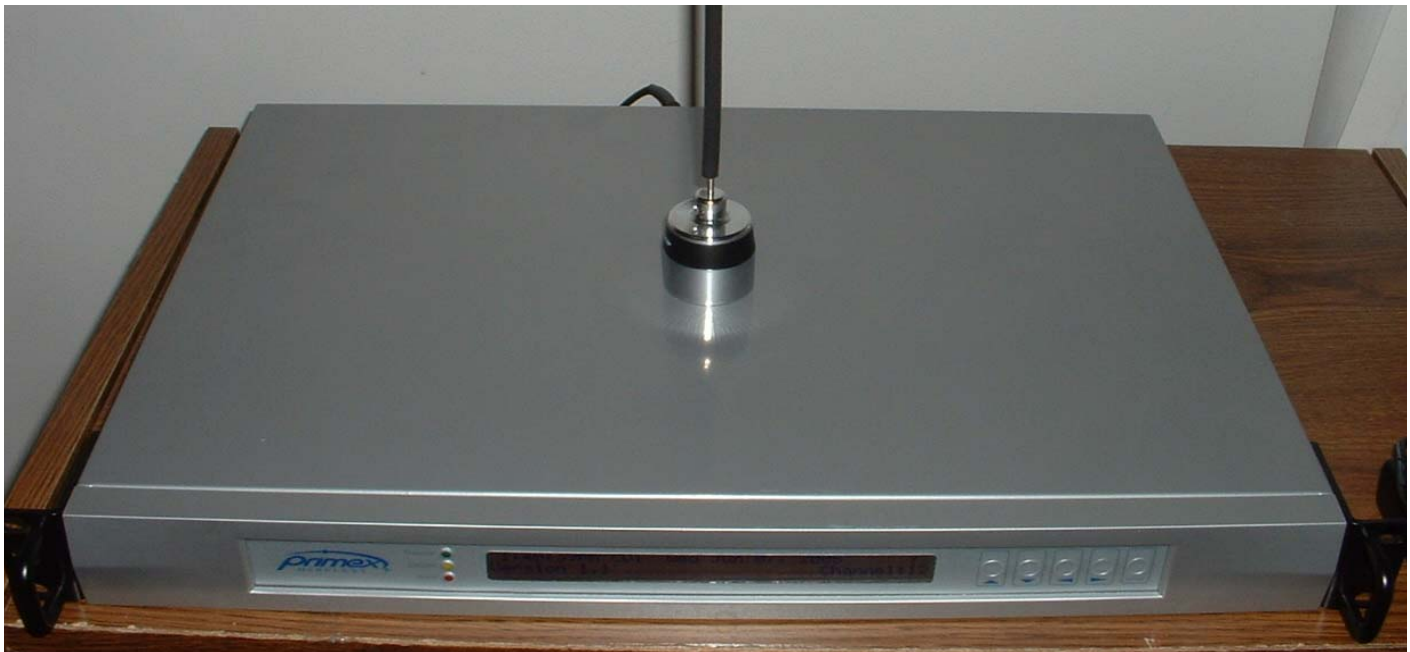
Figure 4 – Overall Picture of XR Transmitter Showing the NMO Antenna Mounted
