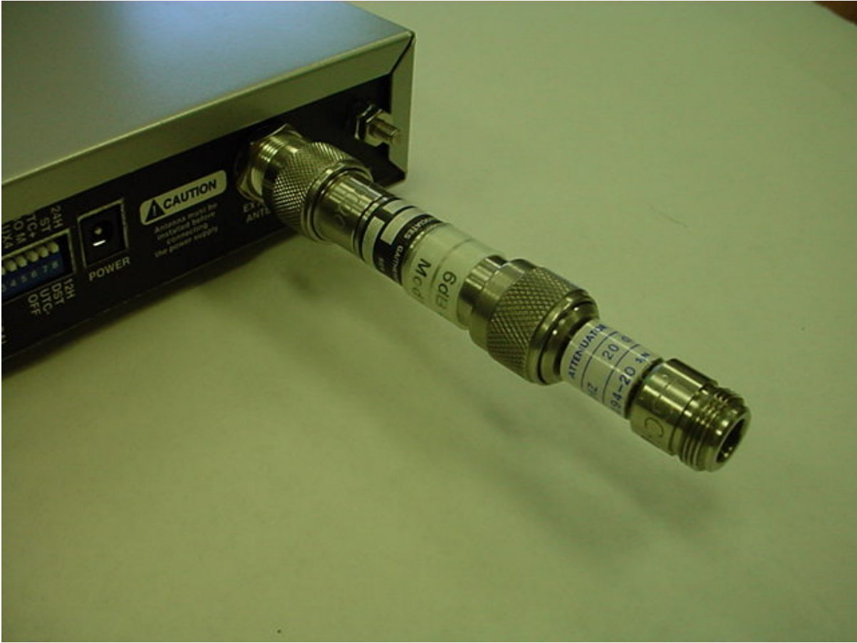
Photo Six – External Antenna Port with Dummy Load for Testing
