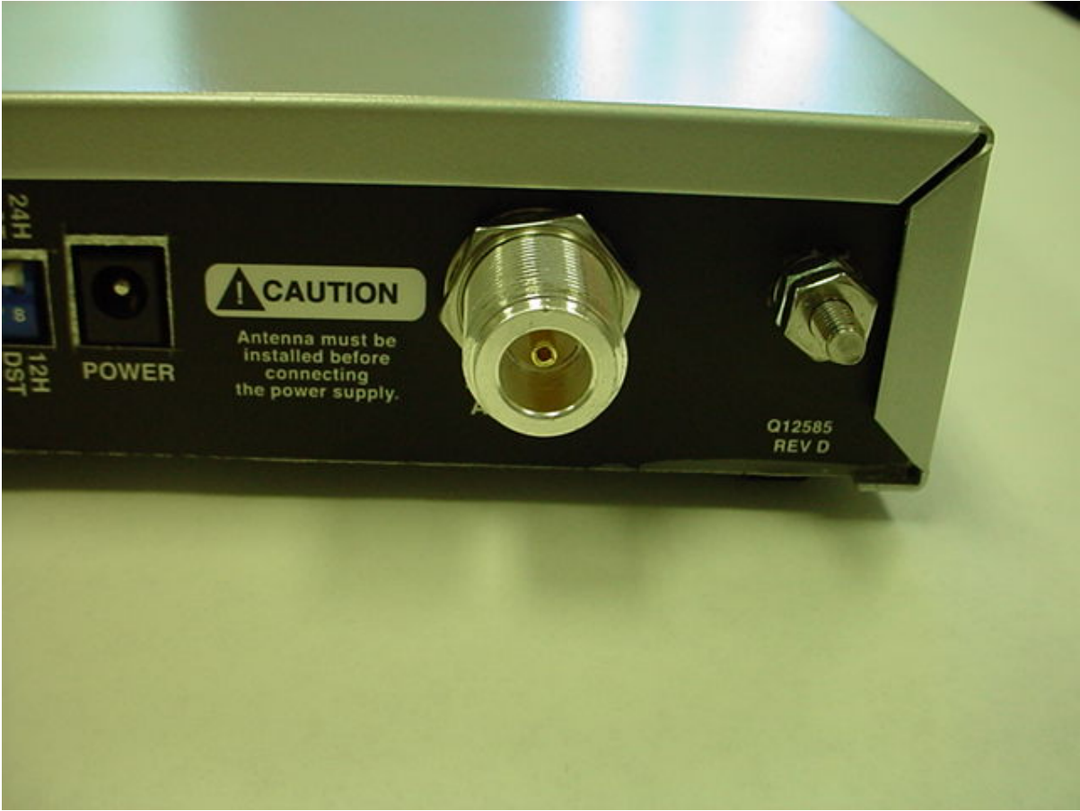
Photo Five – External Antenna Port
