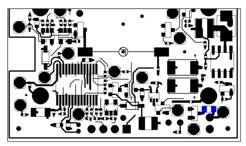
Description of Modification: To suppress the 276MHz harmonic before it reached the power wires and radiate a ferrite bead was added to the board positioned above the positive battery terminal (shown above in blue) directly in line with the positive voltage supply line for the PCB. Adding this Ferrite Bead in this location helps to reduce the 276MHz harmonic from being conducted into the battery wires.
