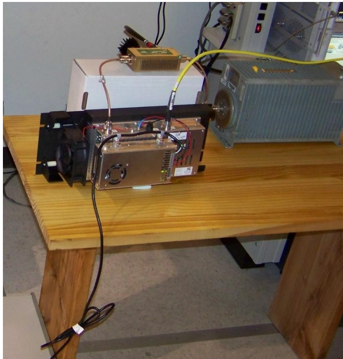
Figure 36: The EUT setup during Spurious RF Emissions Measurements.
