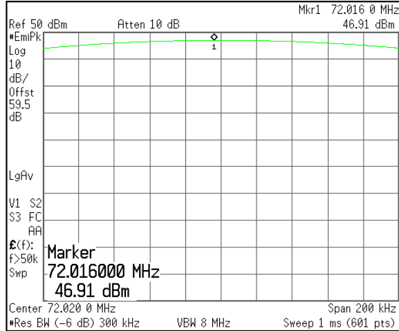
Figure 12: RF Output Power, 72.02 MHz, 50W
