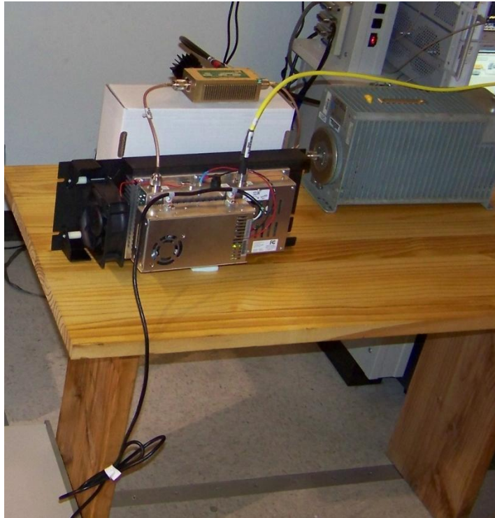
Figure 16: The EUT setup during Occupied Bandwidth tests.
