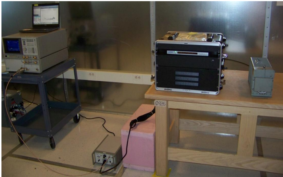
Figure 66: The EUT setup during Conducted RF Emissions tests onto AC Mains.
