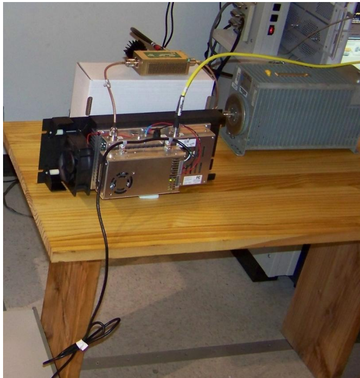
Figure 31: The EUT setup during Band-Edge Measurements.
