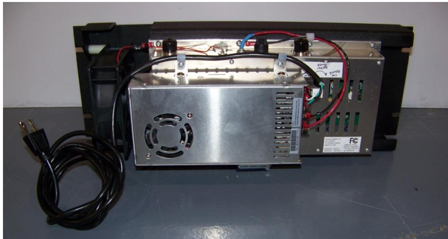
Figure 3: Rear view of the 72XR power amplifier (not exposed to end-user)
