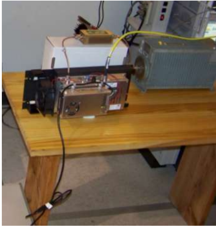
Figure 8: The EUT setup during Occupied Bandwidth tests.
