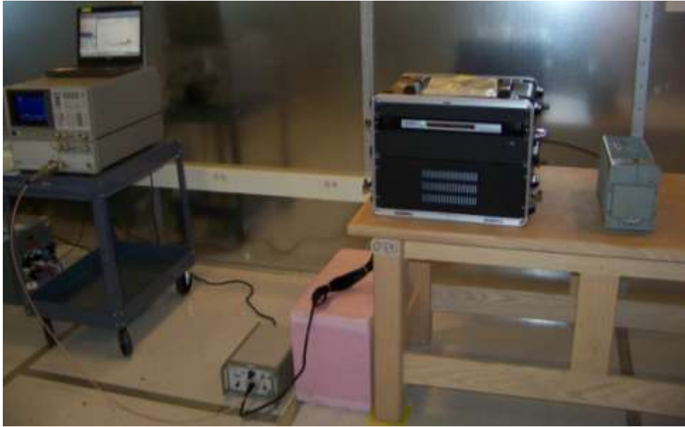
Figure 20: The EUT setup during Conducted RF Emissions tests onto AC Mains.
