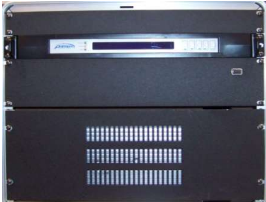
Figure 5: The Command Point 72XR System, as presented to the end-user (includes the power amplifier) Front view.
