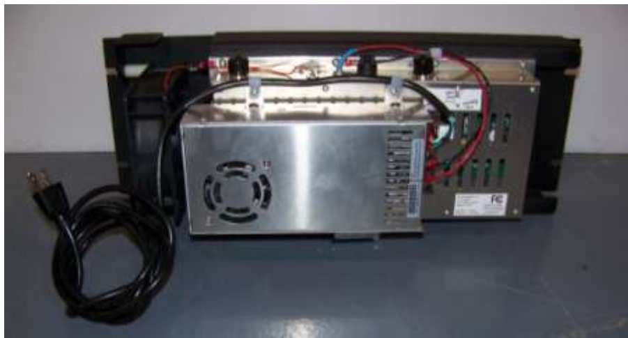
Figure 3: Rear view of the 72XR power amplifier (not exposed to end-user)
