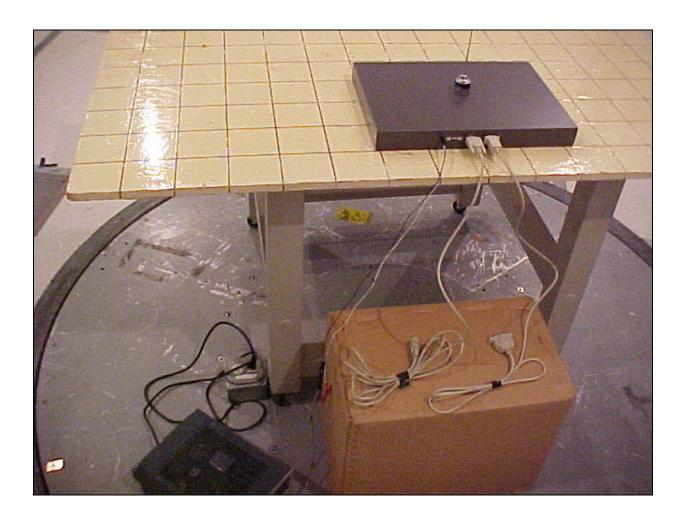
View of the EUT during the <u>Radiated Emissions</u> Testing. Antenna in place, but port internally terminated with a 50 Ohm load.
