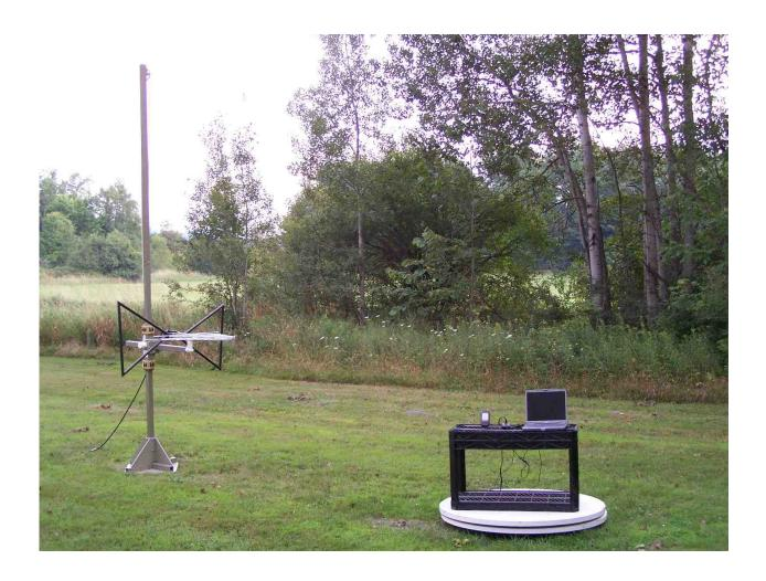
Photograph 1 – Radiated Emissions <1 GHz - FCC ID PYVR63311
