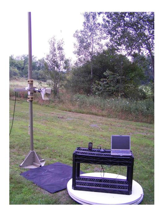
Photograph 2 – Radiated Emissions >1 GHz - FCC ID PYVR63311
