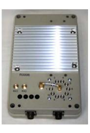
The Ruggedized Reader provides all of the RF and control functions required to power and communicate with Matrics passive RFID tags (PN: SDR-IP-001 and DDS-IP-001.) It sends digital data to the tag (through one antenna at any given time) on a pulse width modulated On Off Keyed (OOK) transmitter signal, demodulates the identification signal received from the tag, and then sends the data to your host computer.
