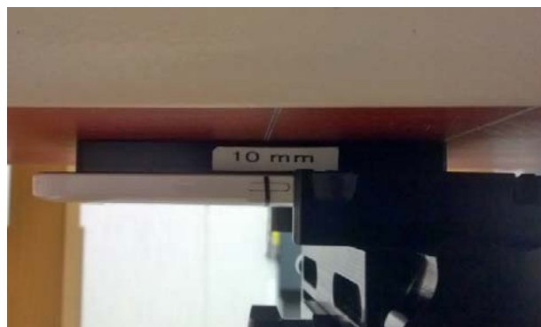
Photo of the device positioned for WR mode measurement – display facing phantom. The spacer was removed before the start of the measurements.
