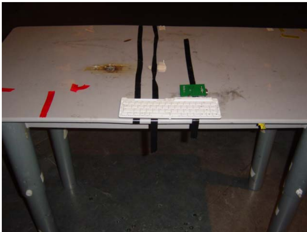
Set-up for Radiation Emission (Transceiver)
