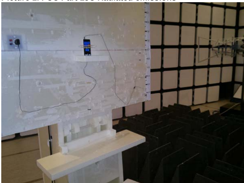
Picture 2. FCC Part 15B Radiated emissions
