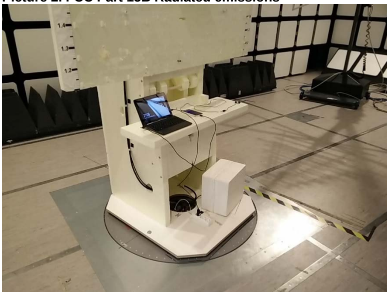
Picture 2. FCC Part 15B Radiated emissions
