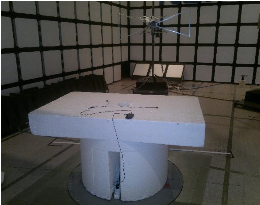
Picture 2. FCC Part 15B Radiated emissions
