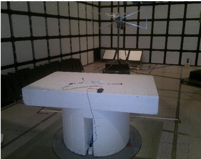
Picture 2. FCC Part 15B Radiated emissions
