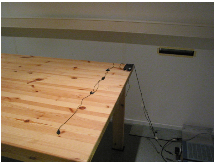
Picture 3 AC powerline conducted emission measurement 15C
