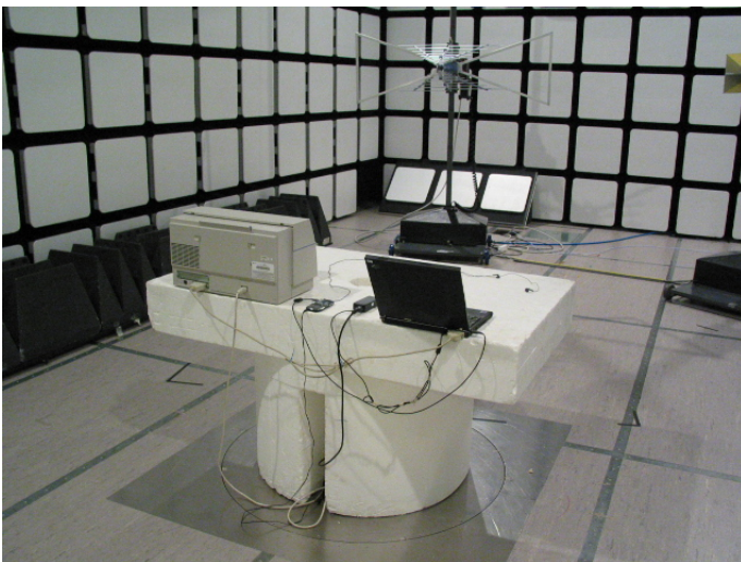
Picture 2 Radiated emission 15B
