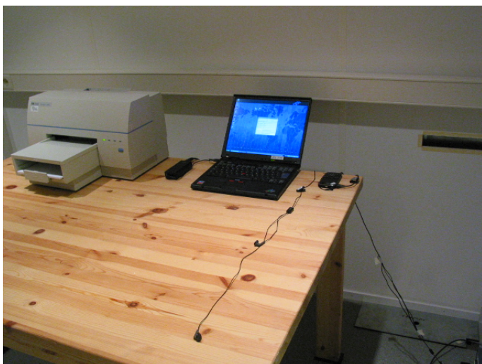
Picture 4 AC powerline conducted emission measurement 15B
