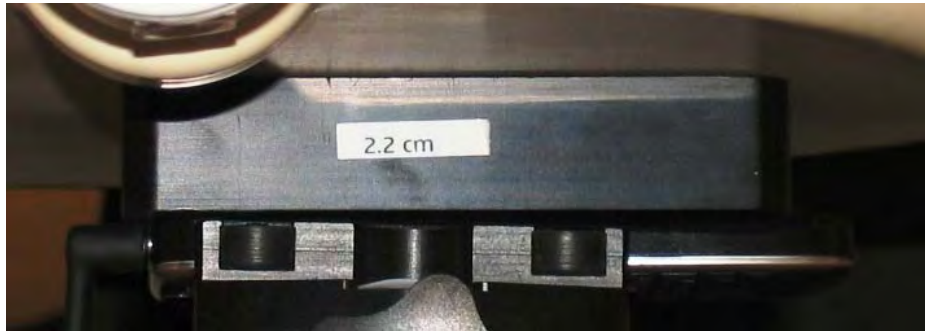
Photo of the device positioned for Body SAR measurement. The spacer was removed for the tests.
