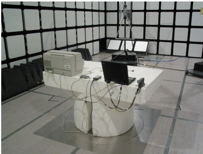
Picture 2 Radiated emission 15B
