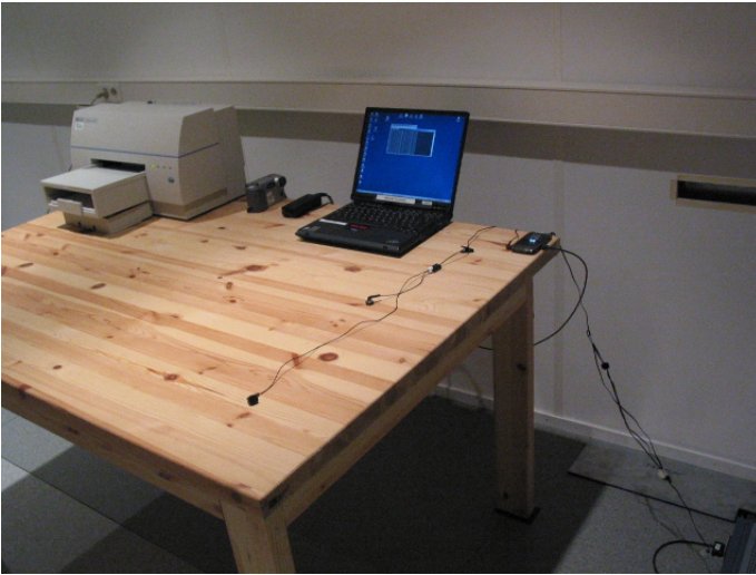
Picture 5 AC powerline conducted emission measurement GSM RX / Bluetooth TX / WLAN RX+ Computer peripherals
