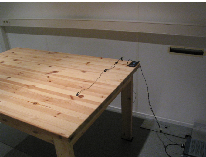
Picture 4 AC powerline conducted emission measurement Bluetooth TX / WLAN TX
