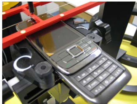
Device positioned under Test Arch
