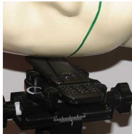
Photo of the device in “tilt” position with slide open
