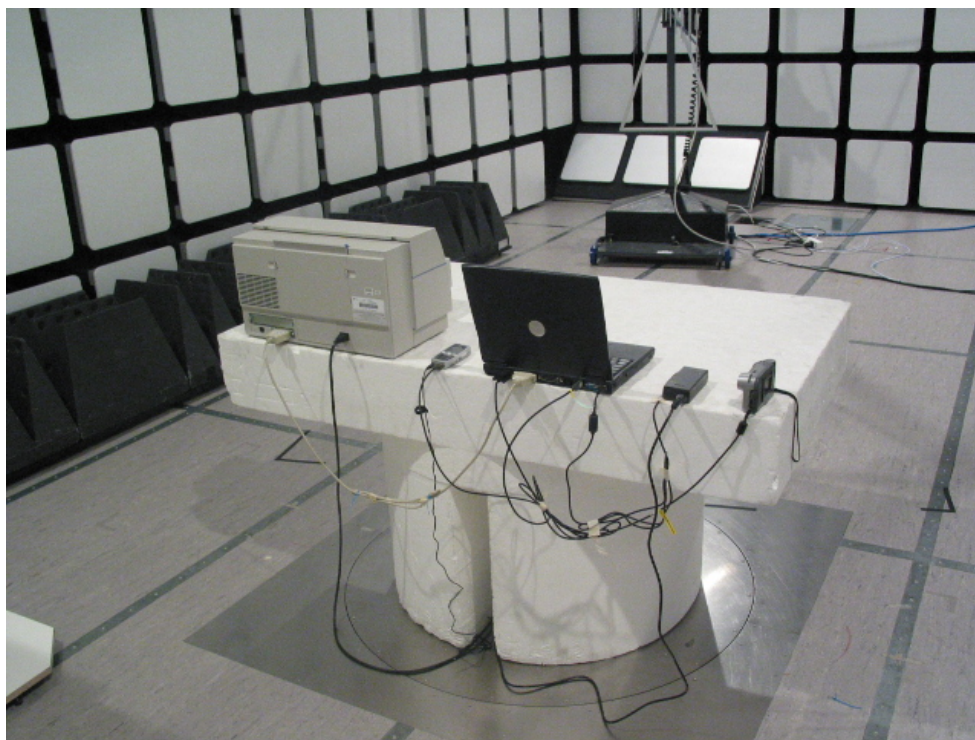
Picture 2 Radiated emission measurement
