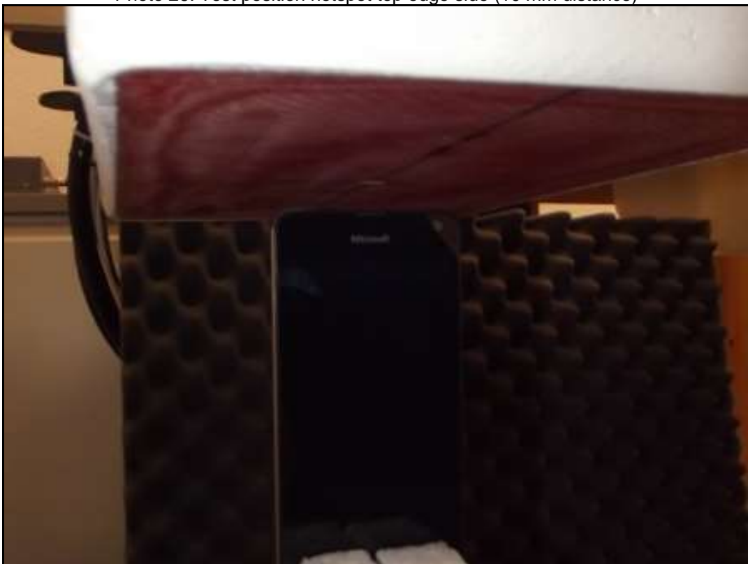
Photo 26: Test position hotspot top edge side (10 mm distance)
