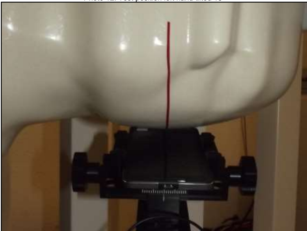
Photo 12: Test position left hand tilted 15°
