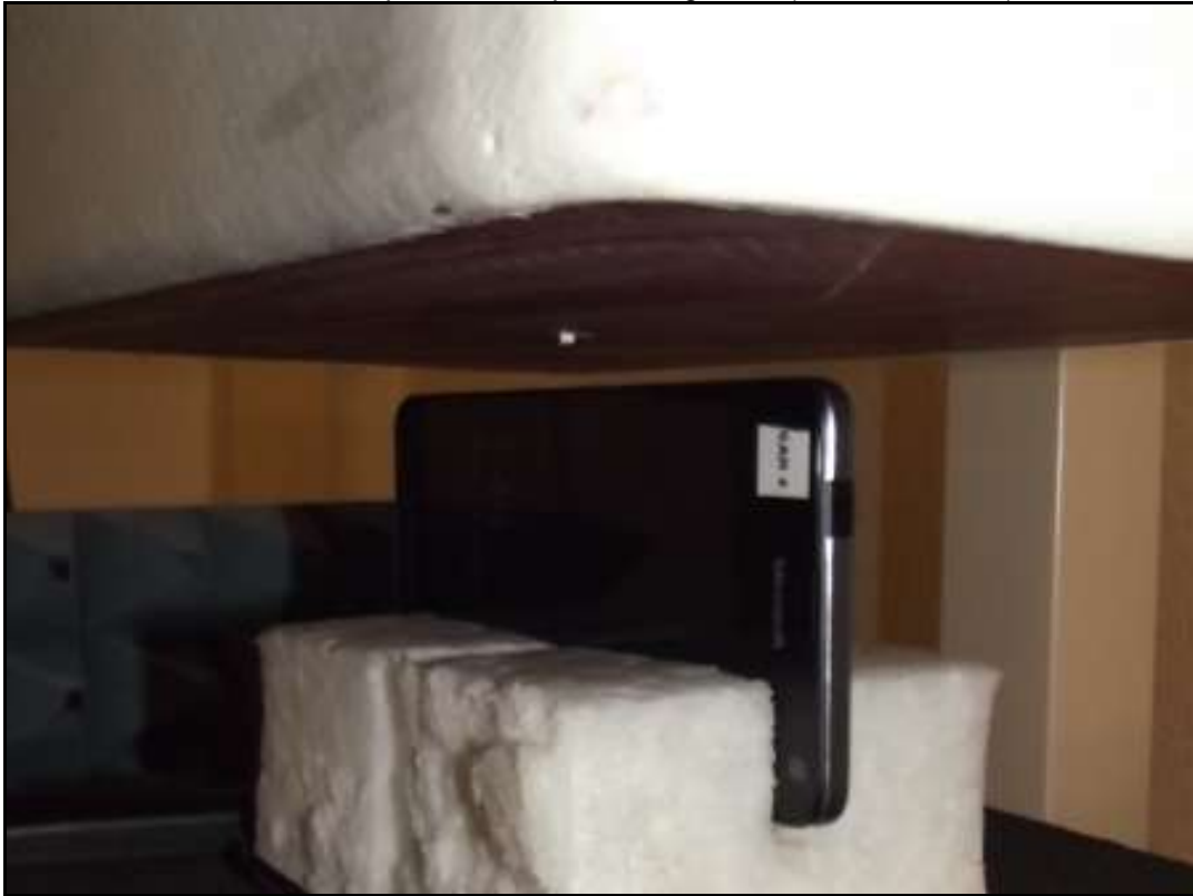
Photo 24: Test position hotspot right edge side (10 mm distance)
