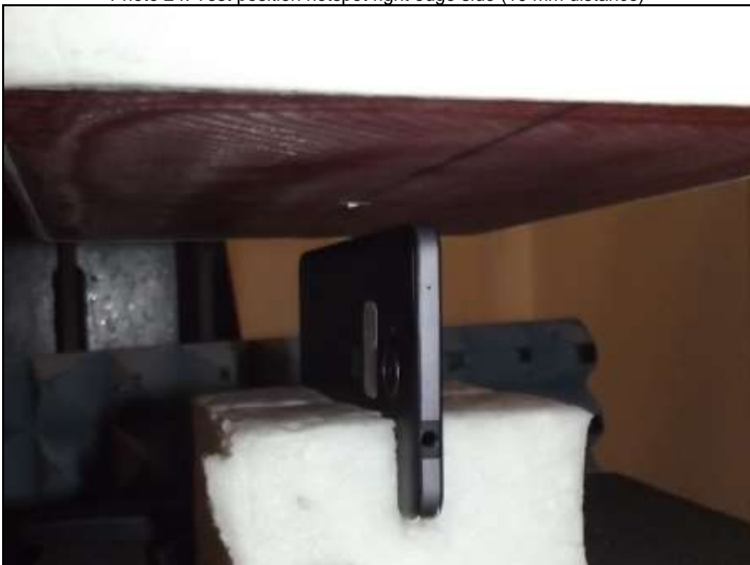
Photo 24: Test position hotspot right edge side (10 mm distance)
