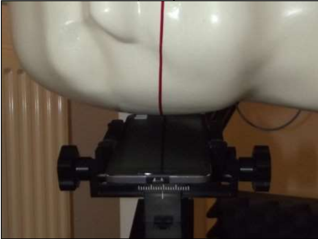
Photo 18: Test position right hand tilted 15°
