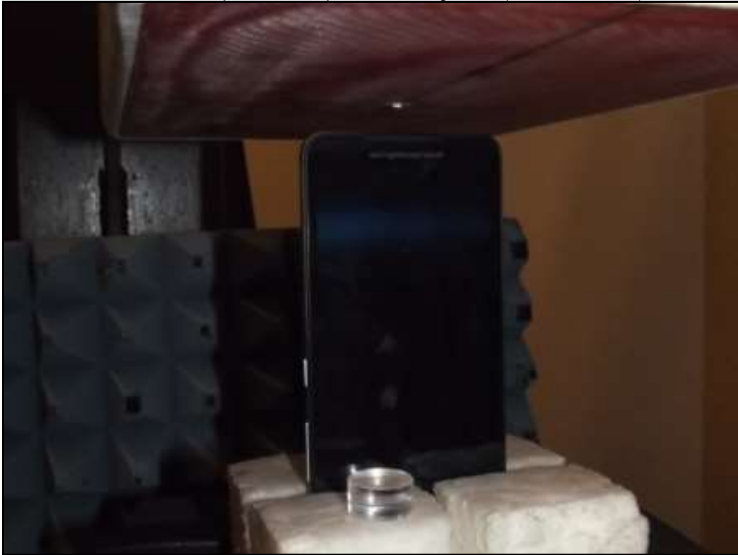
Photo 26: Test position hotspot top edge side (10 mm distance)
