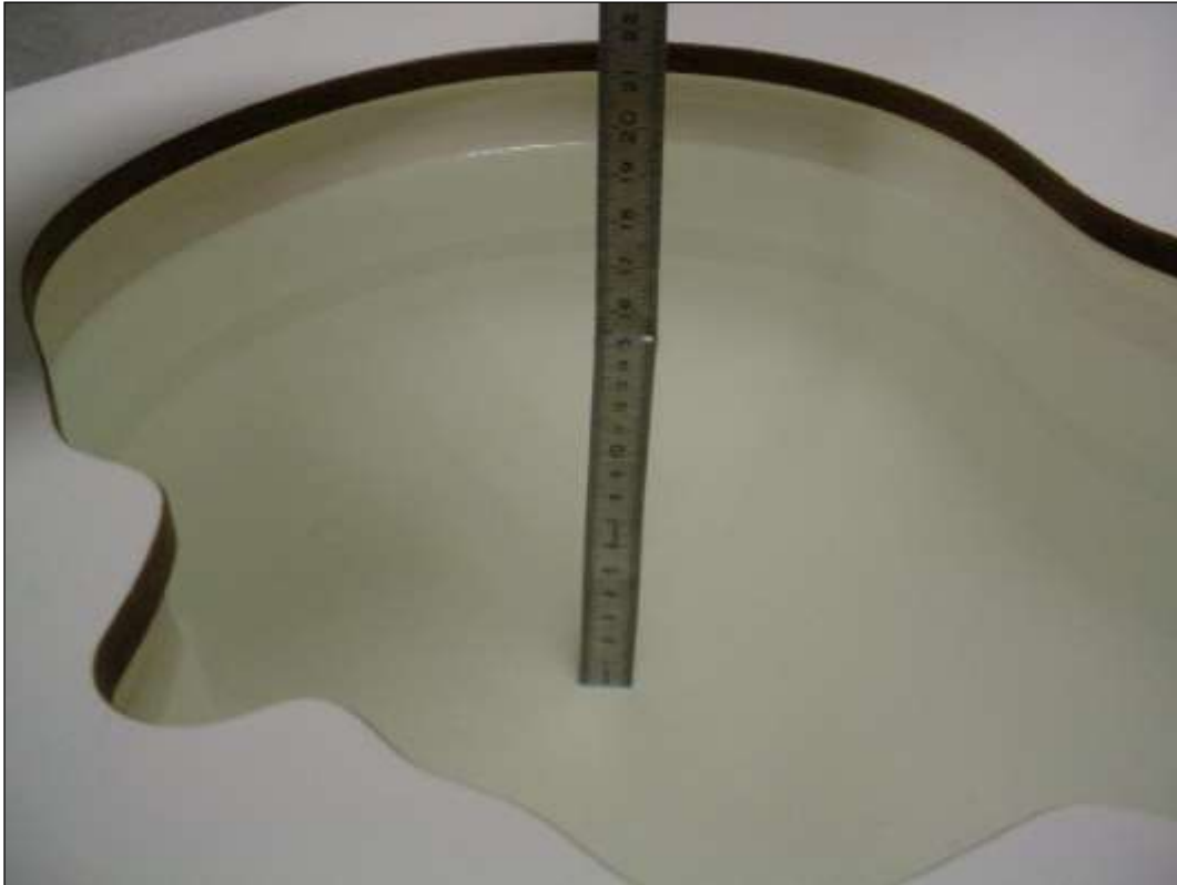
Photo 4: Liquid depth 1750 MHz body simulating liquid
