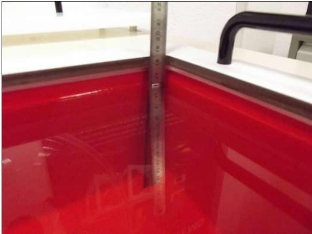
Photo 2: Liquid depth 850 MHz body simulating liquid
