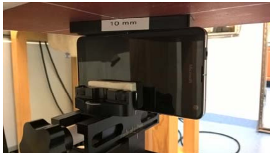
Photo of the device positioned for WR mode measurement – left edge facing phantom. The spacer was removed before the start of the measurements.
