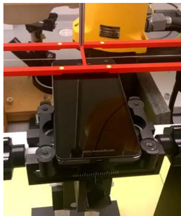
Photo of the device positioned under Test Arch
